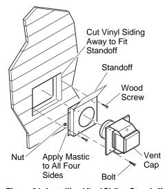
Figure 24 - Installing Vinyl Siding Standoff
